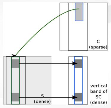
Data layout is SC(16, 16, N/16): All 16x16 matrices are 256-bit aligned and fit in L1 cache. 100% vectorized
