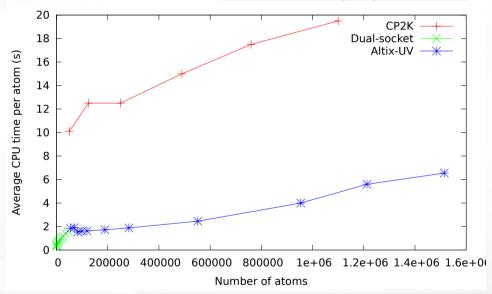
Comparison is not quantitative: different architectures, different method, different number of SCF cycles
