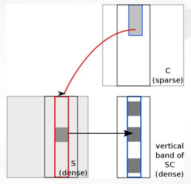
Data layout is SC(16, 16, N/16): All 16x16 matrices are 256-bit aligned and fit in L1 cache. 100% vectorized
